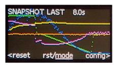
Snapshot screen provides a "black box" view for analysis of crash or any other problem. Records only when the motor is turning, keeping recorded data when the motor is stopped. It is set to record last eight seconds by default but mode can be switched by long press to shorter time or to record first seconds of motor run if you need to analyze acceleration from standstill.
